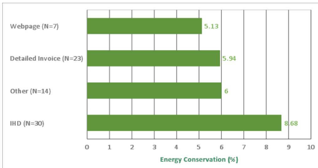
Figure 7: Energy reduction achieved through different customer feedback mechanisms
