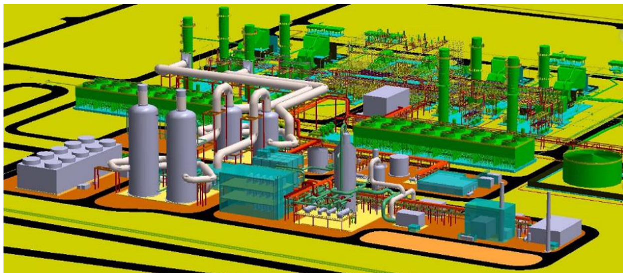
Fig. 20: 3D view of a gas-fired combined cycle power plant with Siemens PostCap™ Plant with two absorption lines
