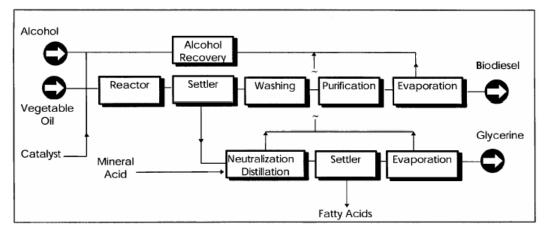
Although the trans-estherification process doesn't imply a complicated chemical reaction, it is particularly difficult to conduct it properly, which calls for the highest industrial standards to ensure the quality of biodiesel. Today, biodiesel produced or marketed in Europe should meet the specifications of the CEN standard EN 14214.
