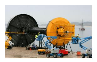
Seabased's Linear Generator has a buoyant surface float attached via a flexible connector to a unit on the sea bed (Fig. 14.8). The movement of the float is converted directly into electricity using a linear generator (such a generator has been used in other devices, such as the most powerful device yet deployed, AWS Ocean Energy's Waveswing). A pilot project of up to 10 x 10 kW devices has been under way in Sweden since 2002.
