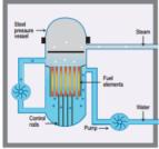
A Boiling Water Reactor (BWR)
