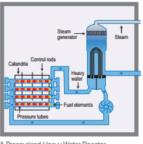
A Pressurized Heavy Water Reactor (PHWR/Candu)
