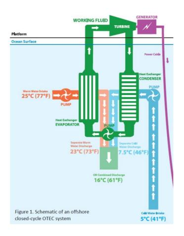
FIGURE 8: OFFSHORE CLOSED-CYCLE OTEC SYSTEM
