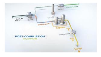
used to capture CO<sub>2</sub> for use in the food and beverage industry. Post-combustion capture processes are integral in both the Boundary Dam CCS and Petra Nova Carbon Capture projects.
