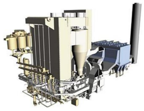
Note: The design by Valmet Power Oy allows great fuel flexibility; the boiler will be able to burn all mixtures of wood and coal from 100% wood to 100% coal. Thermal output is 550 MWth with steam parameters: 194 kg/s,  $165 \, \text{bar}$  and  $545 \, ^{\circ}\text{C}$ .
