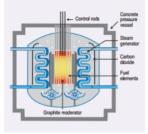
An Advanced Gas-cooled Reactor (AGR)
