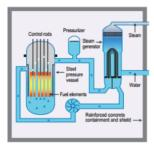
A Pressurized Water Reactor (PWR)
